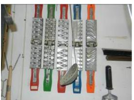
Sinker & Jig Molds
