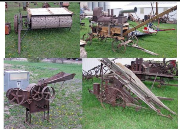
Kentucky Blue Grass Seed Harvester; Several Corn Shellers & Pickers; Hand Shredder; Hand Crank Grain Tester/Cleaner
