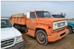
• 1974 Chevy C-60 Single Axle Dump Truck, Gravel Box, Long Block 350 less than 4000 miles on new engine, rebuilt transmission)
