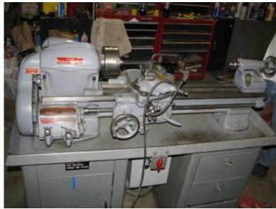
• South Bend Model A Metal Lathe, 3½ Bed, 9" Swing, Quick Change Threads, Reconditioned, Lots of Tooling & Accessories
