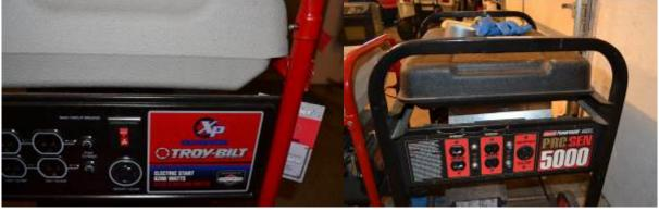
• Generators: TroyBilt 6200 Watt w/ Elec. Start (new) & Coleman Powermate 5000w (rebuilt motor)
