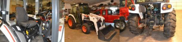
Bobcat Model CT450 4WD Utility Tractor w/ 9TL Bobcat Loader, diesel, 49 HP, 159 hours, all weather cab (heat & AC), comfort seat, farm tires, extra hydraulic hookups (1 front, 2 rear), great shape – nice unit
