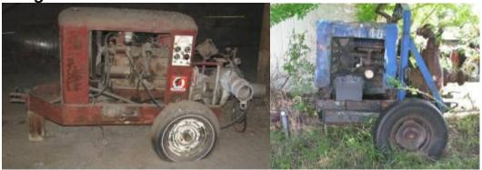
• Choctaw Irrigation Pump w/ Propane Fired Chrysler Industrial Engine
