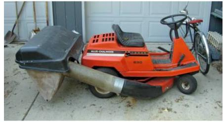
Allis Chalmers 830 Lawn Tractor with Mower/Bagger (was overhauled but air cleaner was loose and sucked in some leaves and scored the piston)
