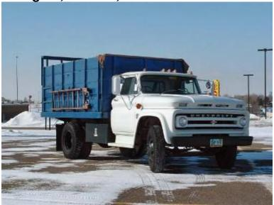
1964 Chevy C-60- 2 Ton Dump Truck, 292 6 Cylinder, 4-Speed w
