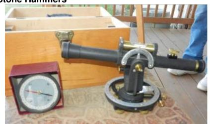
David White Survey Level w/ Survey Compass Attachment, Rod, & Tripod (like new condition)
